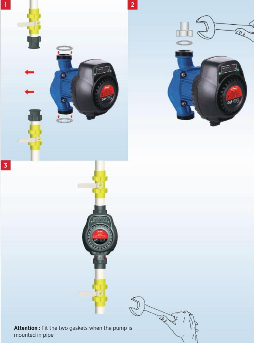
**Attention :** Fit the two gaskets when the pump is mounted in pipe
